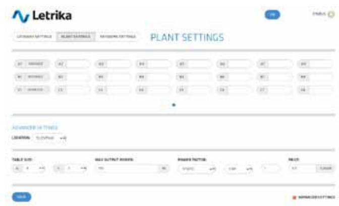
Figure 9: Registering new micro inverters and setting other plant settings
